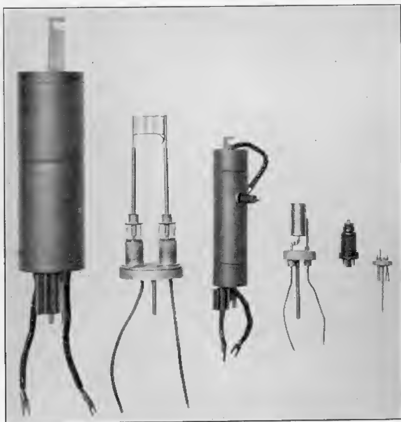
FIG. 86. A group of metal tubes showing the internal structure. At the left is a two-electrode, mercury-vapor tube and cathode header; next, is a shield-grid, mercury-vapor tube and cathode mount and, at the right, a receiving tube and cathode header.
